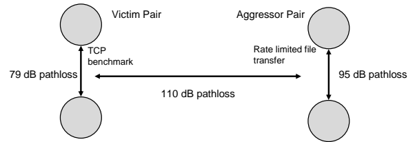
Figure 11: Laboratory Interference Test Topology
