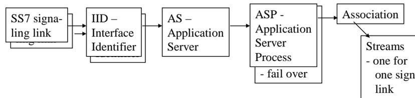
Each signaling link has IID – Interface Identifier
