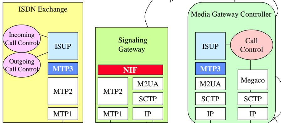
M2UA – MTP2 User Adaptation layer extends MTP2 primitive interface to the IP network: MTP3 of MGC uses SG MTP2 as its layer 2 protocol
