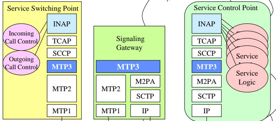
M2PA – MTP2 User Peer-to-Peer Adaptation layer makes IP network look like a signaling channel (including network management features) for MTP3. Carries all the CCS7 signaling network legacy to the IP environment. SCP is an SS7 signaling point. SG = STP in SS7 terms...
