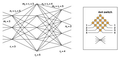
Every SB in stage k is connected to all  $r_{k+1}$  SBs in the following stage k+1 with a single link.
