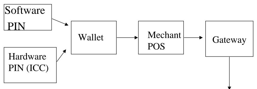
ICC has a small silicon microchip containing Bank 8K to 16K bytes of data. ICC may be capable of generating RSA or ECDSA signatures. POS=point of sale
