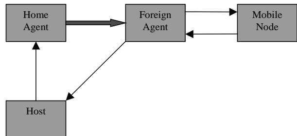
Figure 1: Mobile IP architecture [2]
