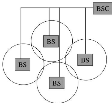
**Figure 3: Cellular network structure**
