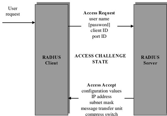
**Figure 5: RADIUS authentication flow [12]**
