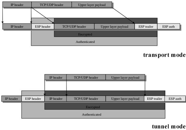
**Figure 2: ESP transformation in tunnel and transport modes**
