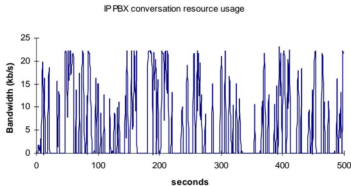
**Figure 15 Usage of resources in IP PBX conversation with G.723 coding**
