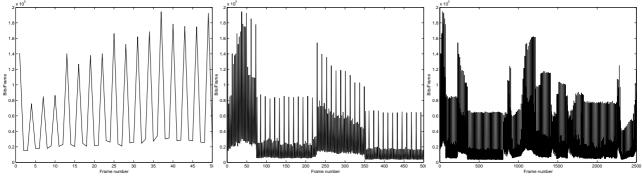
Figure 7: Amount of data in single I, P or B frame. Time of single frame is 33ms.
