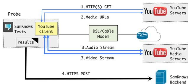
**Fig. 1.** A measurement setup on top of the SamKnows platform. A dual-stacked probe in addition to the standard SamKnows tests, executes the YouTube test. The YouTube test runs every hour and measures a set of performance indicators to endpoints delivering YouTube audio and video both over IPv4 and IPv6. The locally collected measurement results are pushed every hour to the SamKnows data collection server using HTTP.
