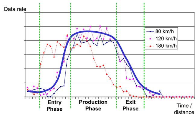
Fig. 2. Different Phases of WLAN Access (UDP)
