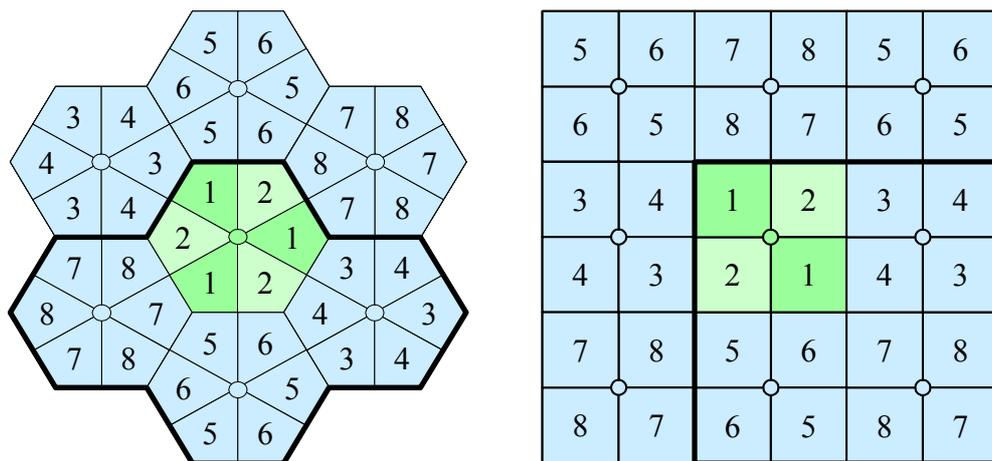
Figure 4.4: Possible frequency reuse patterns using 8 channels
