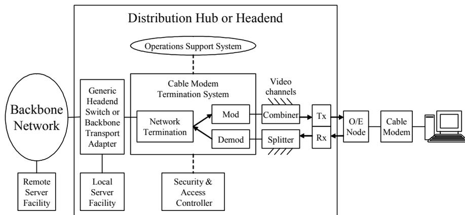
**Figure 2.6: Data-over-cable network architecture (adapted from CableLabs 2002)**
