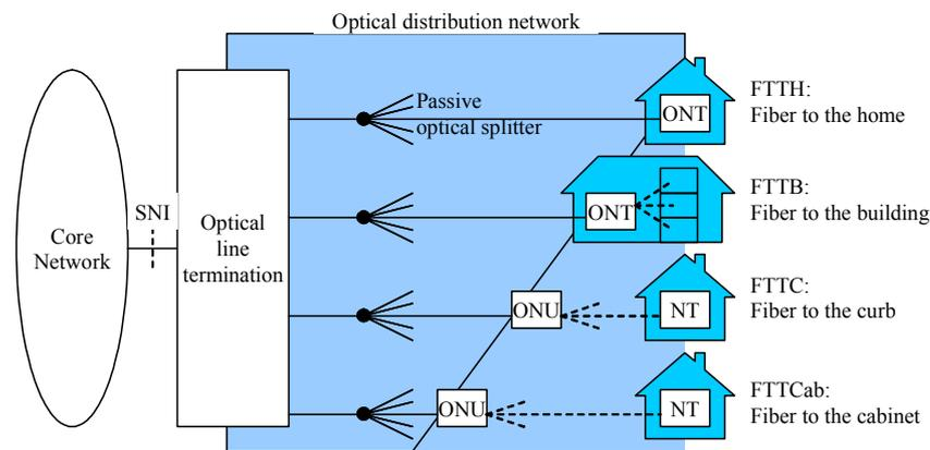
**Figure 2.4: The fiber-to-the-x (FTTx) concept (adapted from Maeda et al. 2001)**
