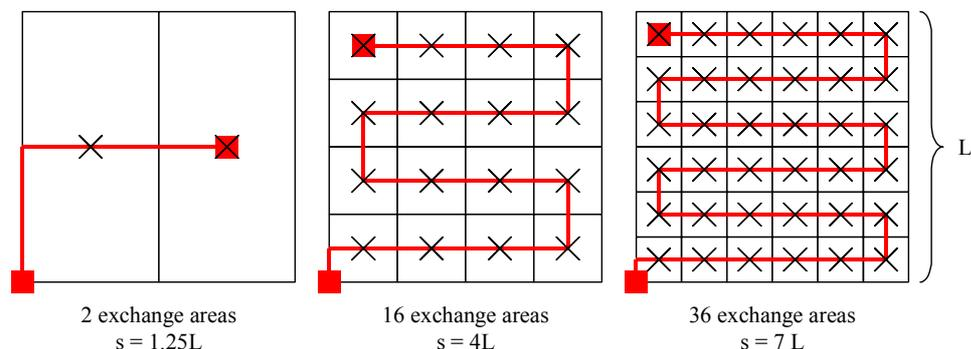
**Figure 6.6: Fiber backbone network dimensioning**
