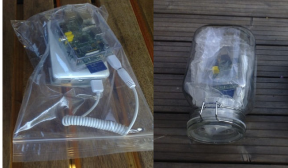
Figure 1: Raspberry Pi hardware in a waterproof container
