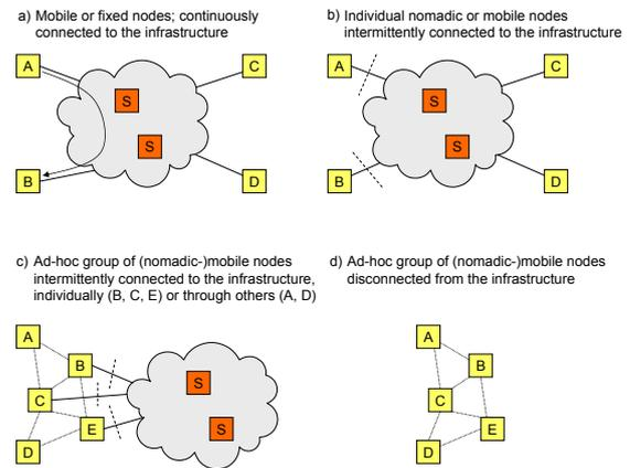
Figure 2: Connectivity variants for mobile nodes
