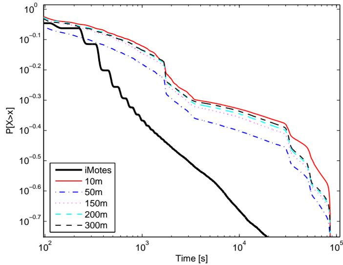
Figure 36: Inter-contact times of additional office size experiments on the Manhattan map
