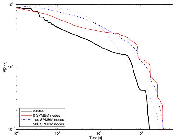
Figure 52: Inter-contact times for different numbers of background SPMBM nodes
