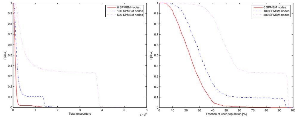
**Figure 54: Total encounters (left) and the fraction of user population encountered (right) for different numbers of background SPMBM nodes**
