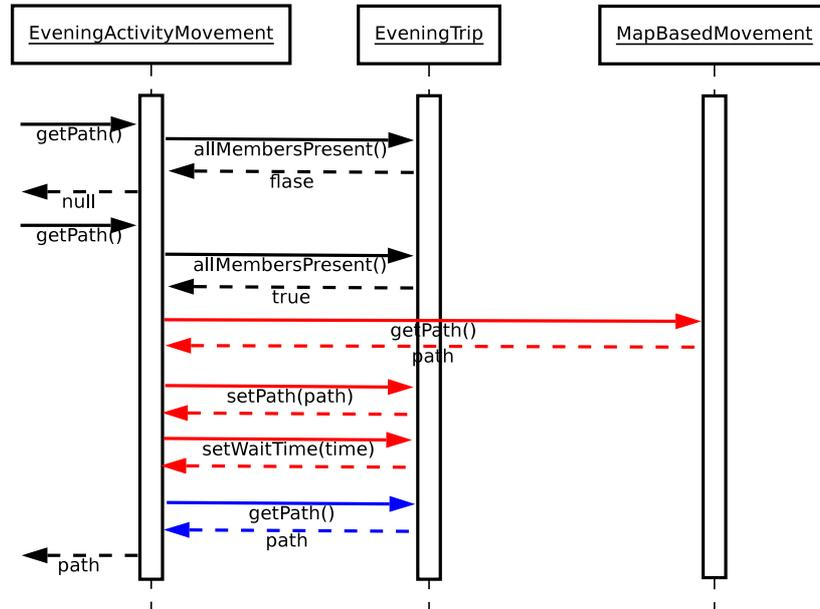
**Figure 11: Sequence diagram of a situation where all nodes are present at a meeting spot and they can start walking in a group. The calls marked in the red color are only made by the first node, while the calls marked in blue color are made by the rest of the nodes.**
