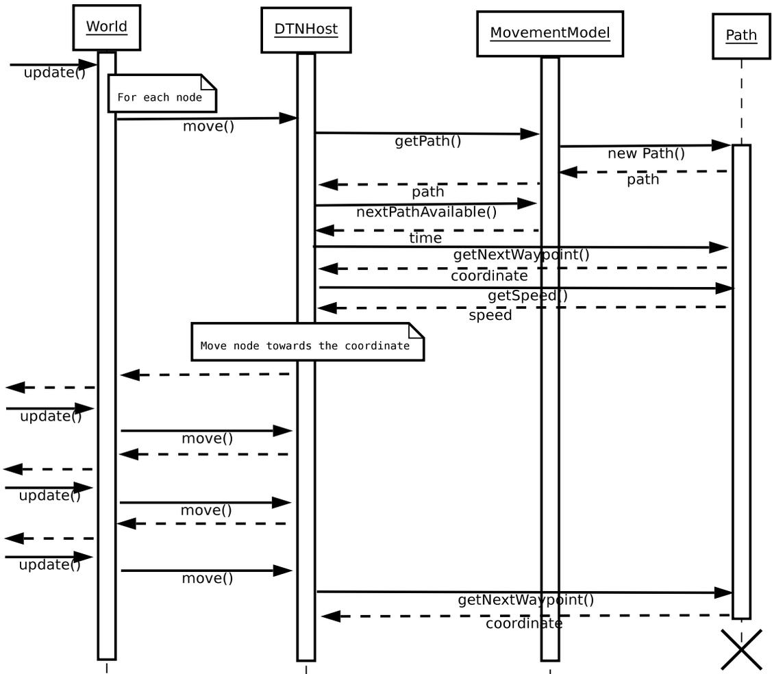
**Figure 6: Sequence diagram of a few update cycles showing how the movement model fits into the big picture.**
