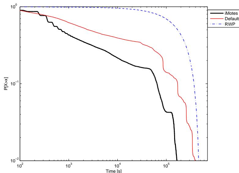
Figure 15: Inter-contact times of Working Day Movement compared to RWP and iMote trace
