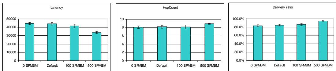
**Figure 57: Performance of the Epidemic routing protocol for different numbers of background SPMBM nodes**
