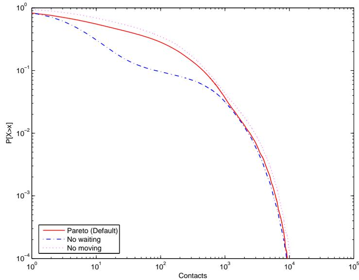
**Figure 41: Number of contacts during an inter-contact time for different pause times inside offices**
