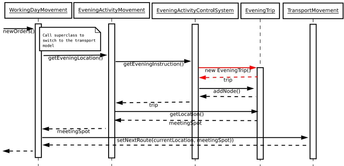
Figure 10: Sequence diagram of a situation right after a node has finished the office activity. The call drawn in red color is only made by the first node in the group.
