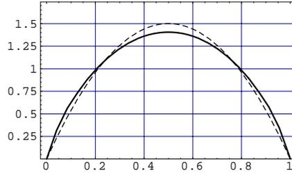
Figure 6: Marginal pdf of the node location in the unit box (solid line) compared with the pdf of the node location in 1-dimensional RWP process (dashed line).
