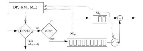
Figure 3 Scheduling and buffering unit of SIMA networking concept
