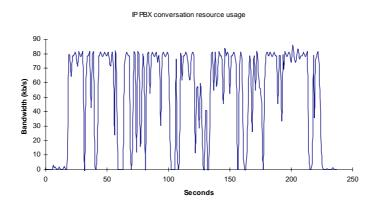
Figure 14 Usage of resources in IP PBX conversation with G.711 coding
