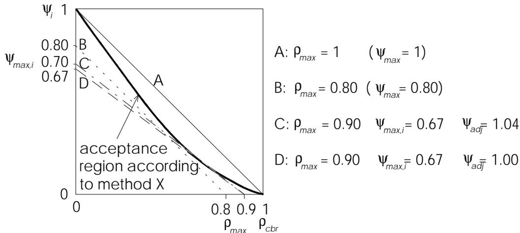
Figure 5.2. The regulating parameters of EB<sub>1</sub> methods (cases A and B) and EB<sub>2</sub> methods (cases C and D).
