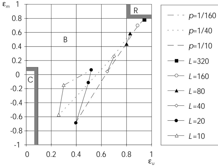
Figure 4.9. Source position on the scale factor plane as a function of  $p_{burst}$  and burst size  $L$ ;  $h = 1/5$ ,  $K = 100$ ,  $P_{loss} = 10^{-4}$ ; C: cell scale, B: burst scale, R: rate-variation scale.
