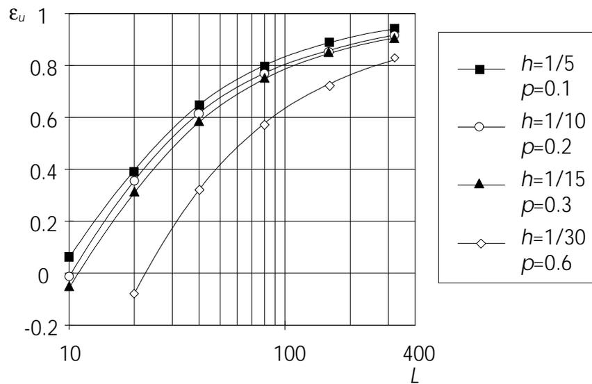
Figure 4.5. Utilisation factor  $\epsilon_u$  as a function of burst size  $L$  for different peak rates  $h$ ;  $m = 1/50$ ,  $K = 100$ ,  $P_{loss} = 10^{-4}$ .
