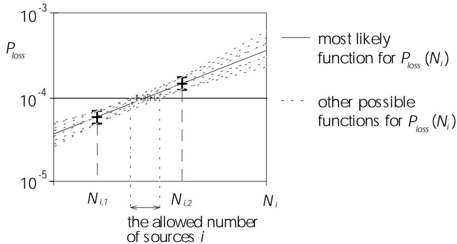
Figure C.1. The accuracy of determination of the allowed number of sources.
