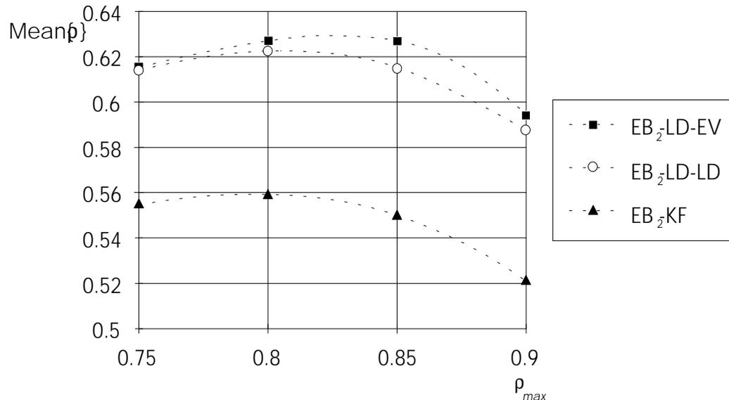
Figure 5.5. The average allowable load as a function of  $\rho_{max}$  for EB<sub>2</sub> methods.
