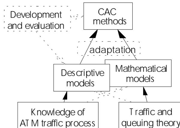
Figure 1.1. A structure for developing Connection Admission Control (CAC) methods.
