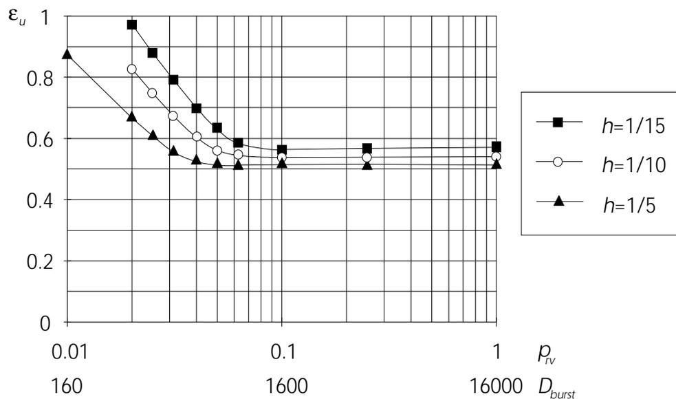
Figure 4.14. Utilisation factor ( $\epsilon_u$ ) as a function of  $p_{rv}$  for three peak rate values;  $L = 20$ ,  $m = 1/800$ ,  $K = 100$ ,  $P_{loss} = 10^{-4}$ .
