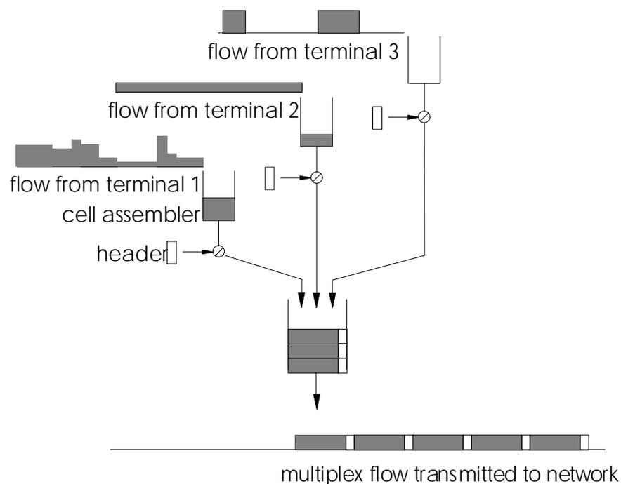
Figure 2.1. The multiplex principle of ATM networks.
