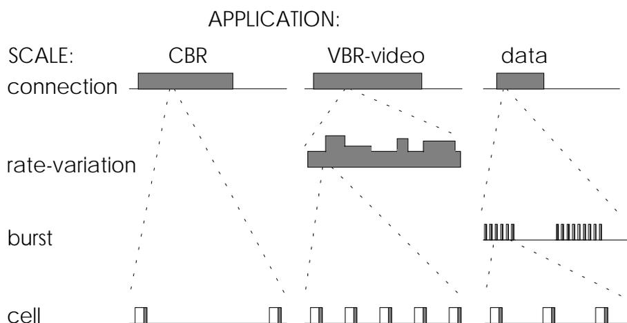
Figure 2.2. Time resolution of ATM traffic process.
