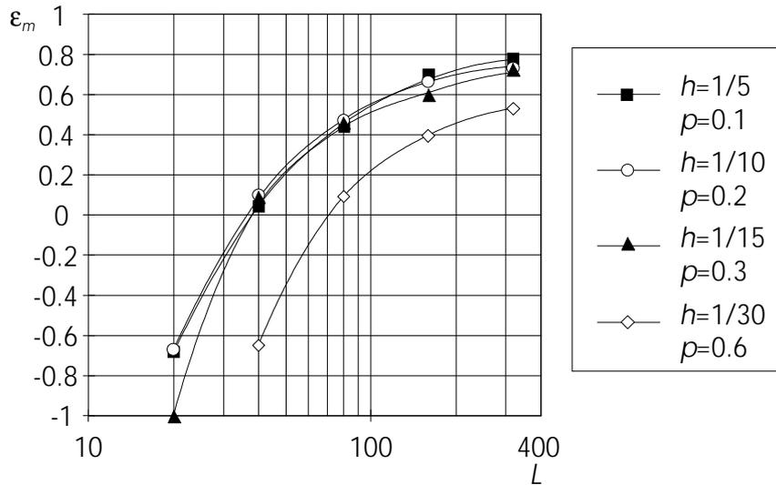
Figure 4.6. Multiplexing factor  $\epsilon_m$  as a function of burst size  $L$  for different peak rates  $h$ ;  $m = 1/50$ ,  $K = 100$ ,  $P_{loss} = 10^{-4}$ .
