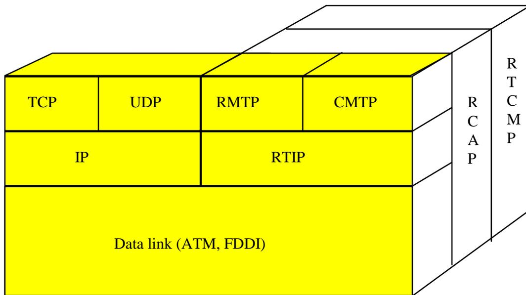
**Figure 18: The Tenet real-time protocol suite.**
