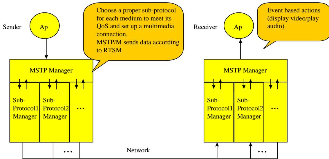
**Figure 3: The architecture of MSTP.**
