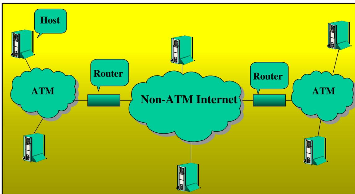
**Figure 23: The IIS network architecture**
