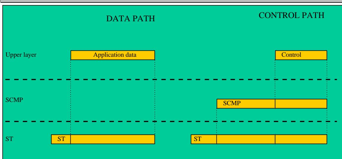
**Figure 13: ST-2 data and control path**
