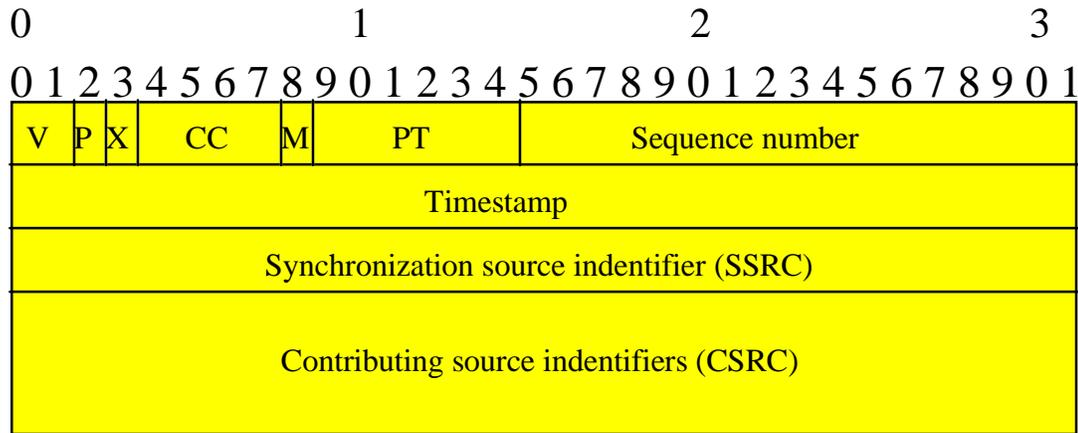
Figure 8: RTP header [4]
