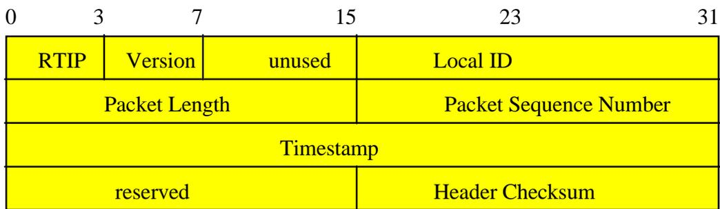
**Figure 19: RTIP packet header**
