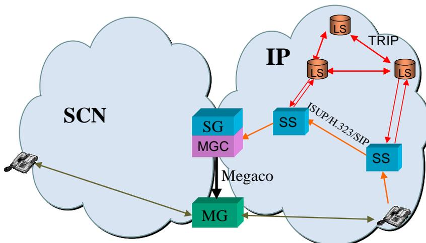
TRIP = Telephony Routing over IP, SG - Signalling Gateway, MGC - Media Gateway Controller
