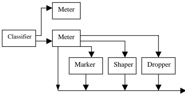
**Figure 2: Structure of an edge device**
