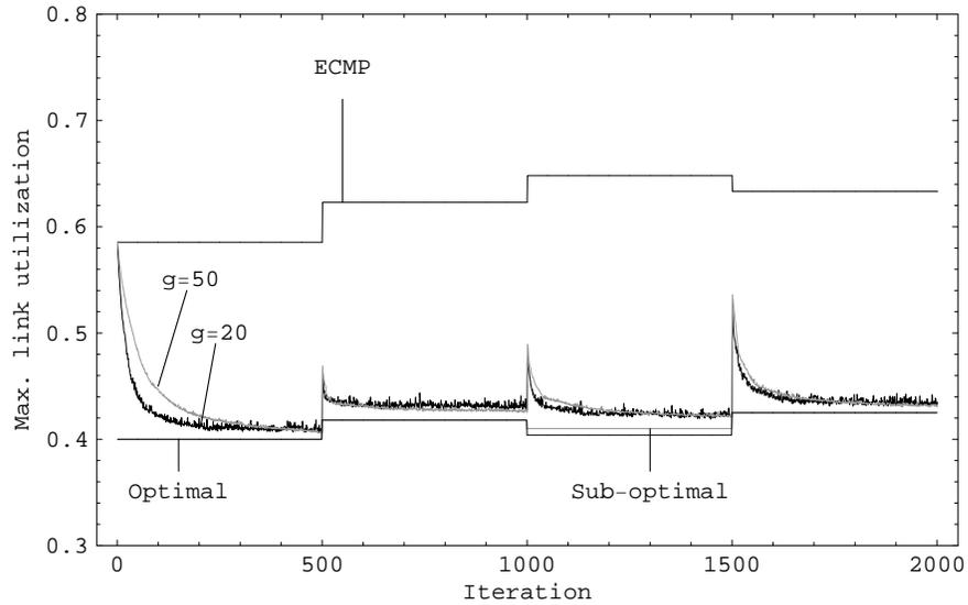
Figure 5.7: The maximum link utilization as a function of the number of iterations, when there are traffic fluctuations at a longer time scale. 20-node network.
