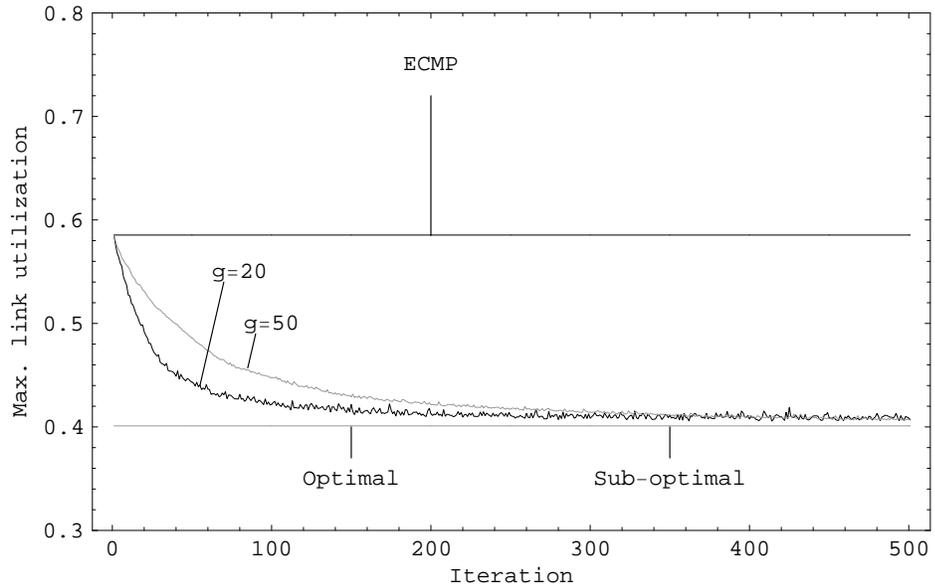
Figure 5.3: The maximum link utilization as a function of the number of iterations, when there are no traffic fluctuations,  $\delta = 0$ . 20-node network.
