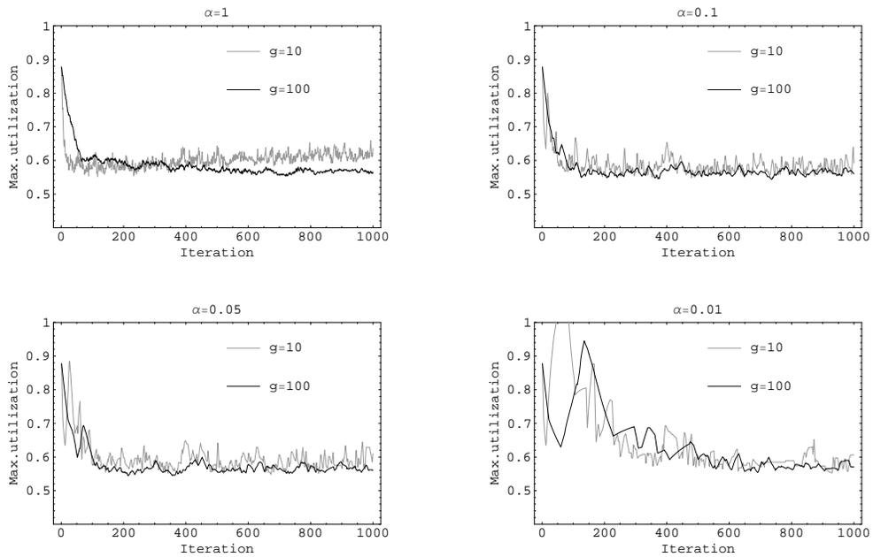
Figure 4.16: The maximum link utilization of variant MINCST combined with EWMA in the 10-node network as a function of the number of iterations.
