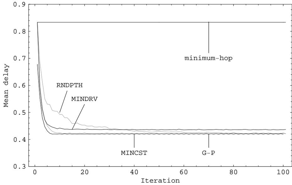
Figure 4.13: The total mean delay in the 15-node network as a function of the number of iterations for the variants RNDPTH, MINCST, and MINDRV of the adaptive load balancing algorithm with granularity  $g = 10$  together with the G-P algorithm.
