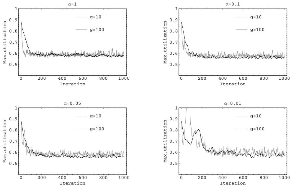
Figure 4.15: The maximum link utilization of variant RNDPTH combined with EWMA in the 10-node network as a function of the number of iterations.
