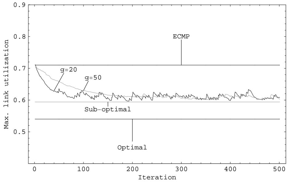
Figure 5.4: The maximum link utilization as a function of the number of iterations, when there are random traffic fluctuations at a shorter time scale,  $\delta = 0.1$ . 10-node network.
