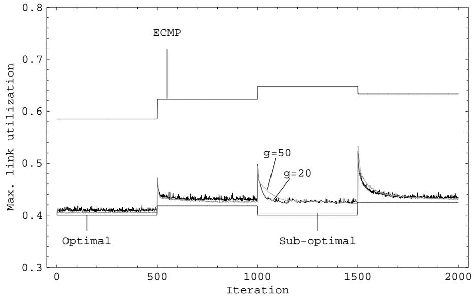
Figure 5.9: The maximum link utilization as a function of the number of iterations. 20-node network.
