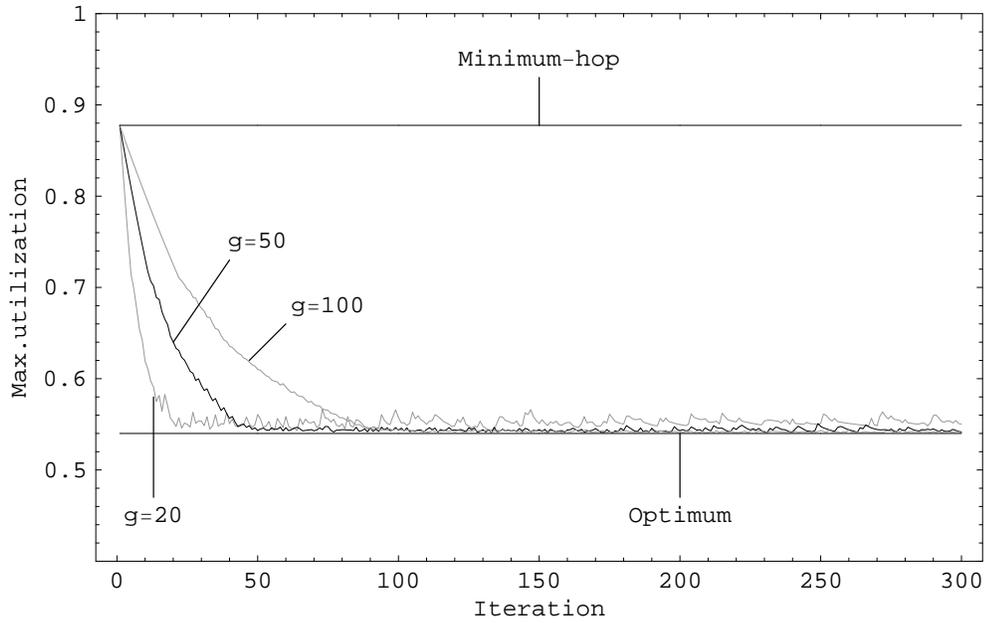
Figure 4.9: The maximum link utilization in the 10-node network as a function of the number of iterations for different levels of granularity  $g$ . Variant MINCST.
