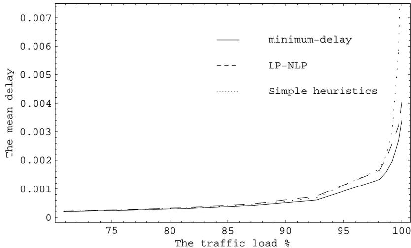
Figure 4.4: The mean delay as a function of traffic load. Granularity parameter in the simple heuristics is  $g = 128$ .
