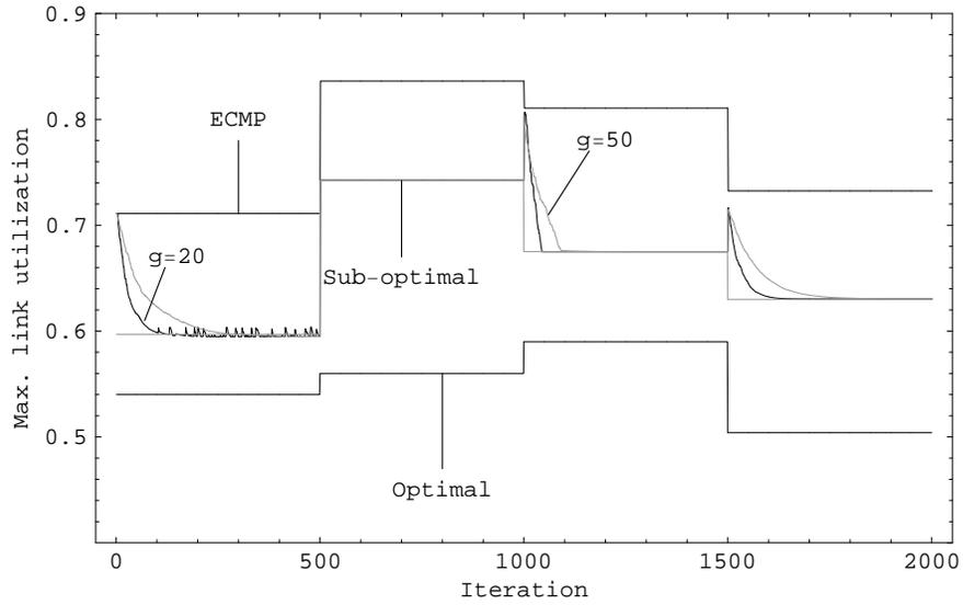
Figure 5.6: The maximum link utilization as a function of the number of iterations, when there are traffic fluctuations at a longer time scale. 10-node network.
