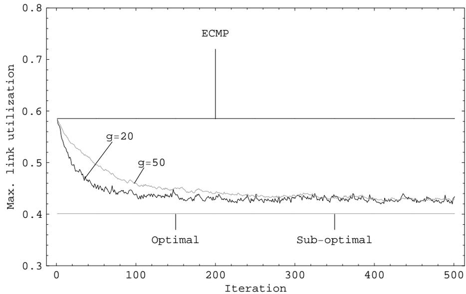
Figure 5.5: The maximum link utilization as a function of the number of iterations, when there are random traffic fluctuations at a shorter time scale,  $\delta = 0.1$ . 20-node network.
