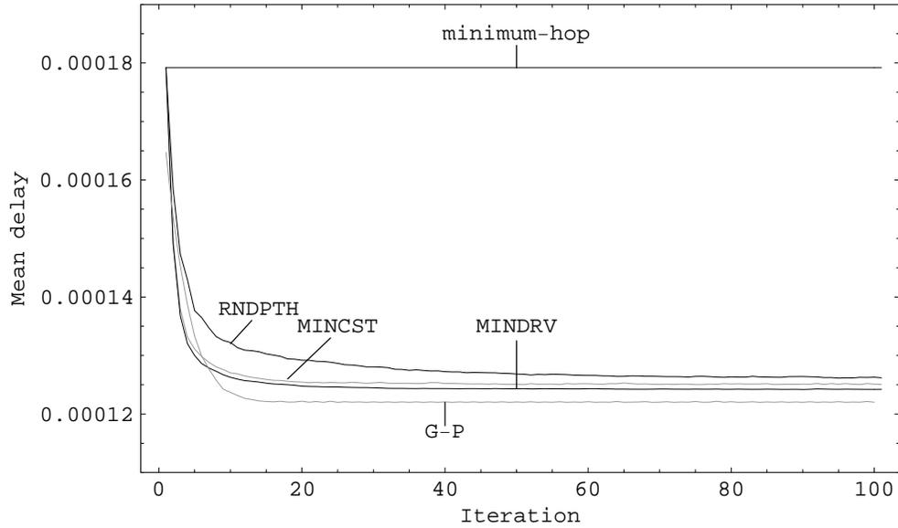
Figure 4.12: The total mean delay in the 10-node network as a function of the number of iterations for the variants RNDPTH, MINCST, and MINDRV of the adaptive load balancing algorithm with granularity  $g = 10$  together with the G-P algorithm.
