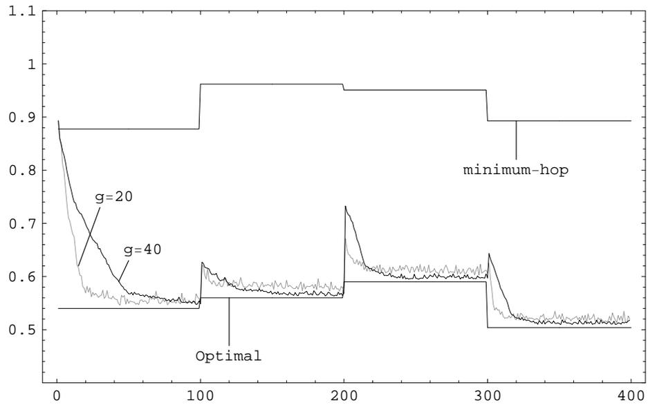
Figure 4.17: The maximum link utilization of variant RNDPTH in the 10-node network as a function of the number of iterations.
