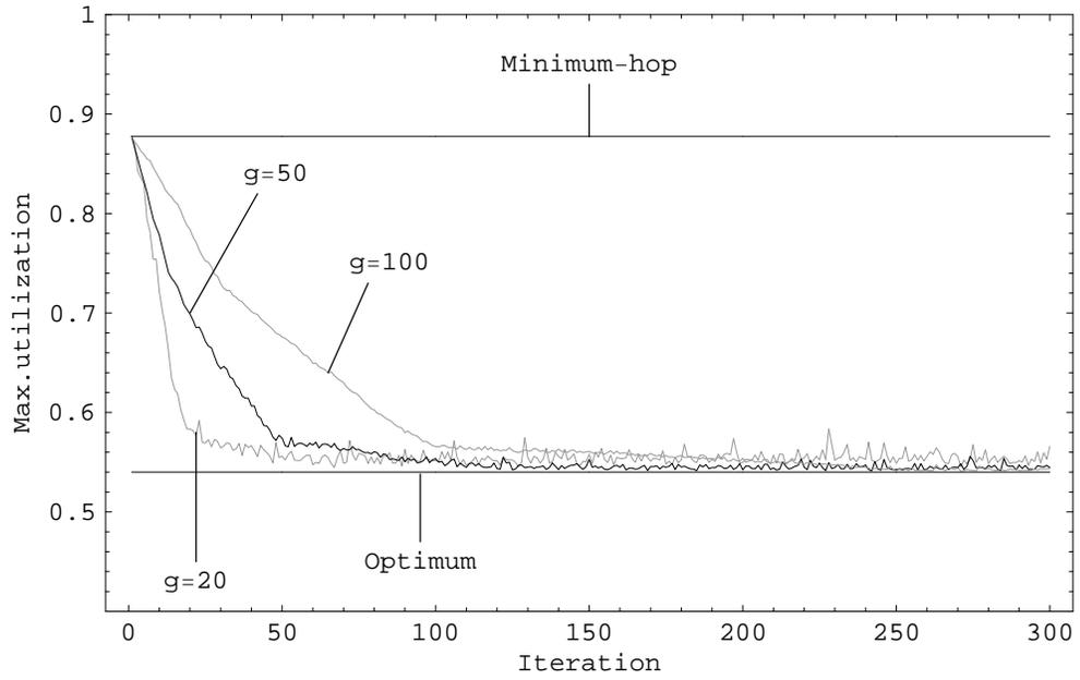
Figure 4.8: The maximum link utilization in the 10-node network as a function of the number of iterations for different levels of granularity  $g$ . Variant RNDPTH.
