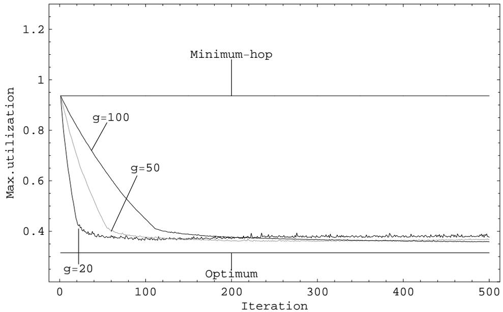
Figure 4.11: The maximum link utilization of variant RNDPTH as a function of the number of iterations for different levels of granularity  $g$ . 20-node network.
