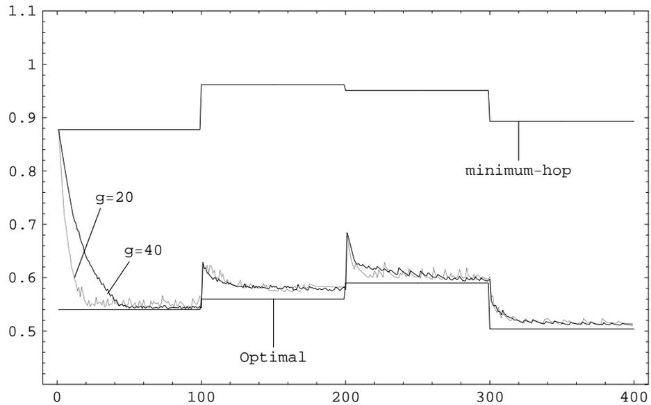
Figure 4.18: The maximum link utilization of variant MINCST in the 10-node network as a function of the number of iterations.
