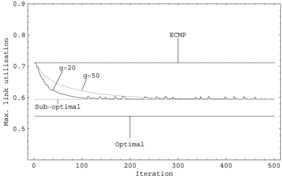
Figure 5.2: The maximum link utilization as a function of the number of iterations, when there are no traffic fluctuations,  $\delta = 0$ . 10-node network.
