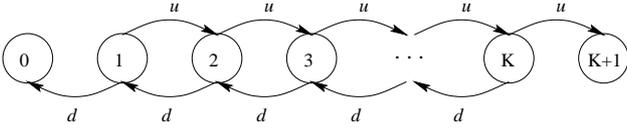
**Figure 1.** Embedded Markov chain of the M/M/1/K-queue.
