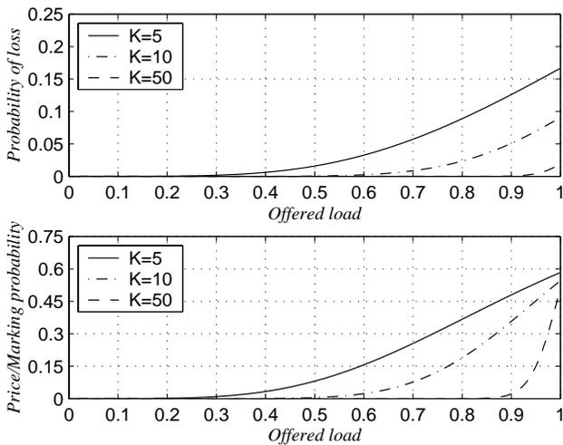
**Figure 4.** Flow level behaviour of the pricing in an M/M/1/K model.
