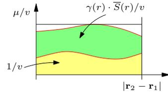
Fig. 6. Averaged sample path realisation for a leg  $\mathbf{r}_1 \rightarrow \mathbf{r}_2$ . The (mean) time spent in each small interval of length  $dr$  is a sum of two components.
