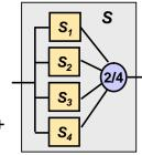
• If  $R_1$ =0.9 , $R_2$ ,=0.95 , $R_3$ =0.85 and  $R_4$ =0.8 then  $R_s$  = 0.994 and  $F_s$  = 0.0058
