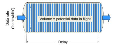
Examples: DVB-S2 geostationary satellite @ 90 Mbit/s x 250ms delay = ~2.8 MB Fiber optic transatlantic link @ 10 Gbit/s x 25ms delay = ~31 MB
