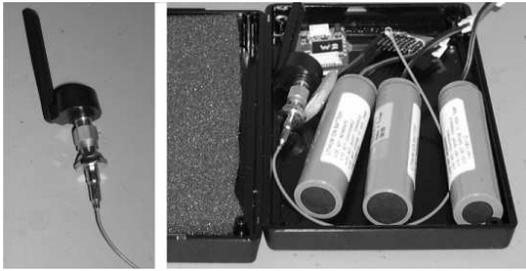
Figure 2: Long range iMote with rechargeable batteries.
