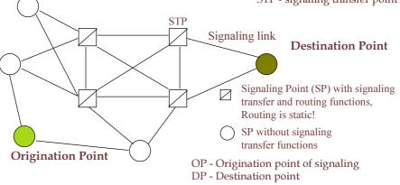
Examle: In Finnish CCS7 no specialized STP -nodes were originally deployed. STP functions were integrated in exchanges. E.g in USA, specialized STP-nodes are commonplace. A use case of STPs is for concentrating IN signaling traffic towards IN nodes that provide Nationwide services.
