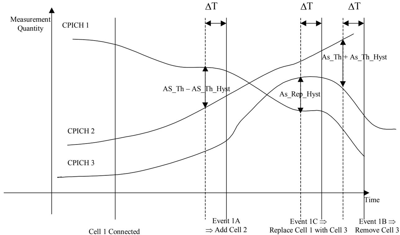
Figure of window-average algorithm from 3GPP 25.922\_3/02
