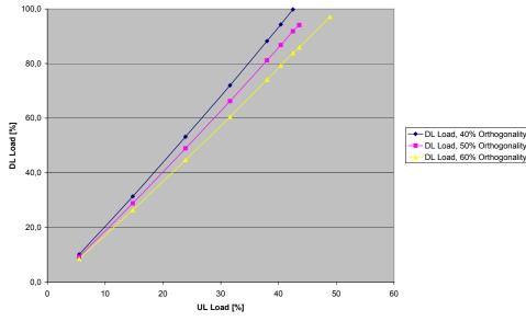
For a given maximum UL load, the greater orthogonality allows for higher tolerable path loss, meaning more coverage
