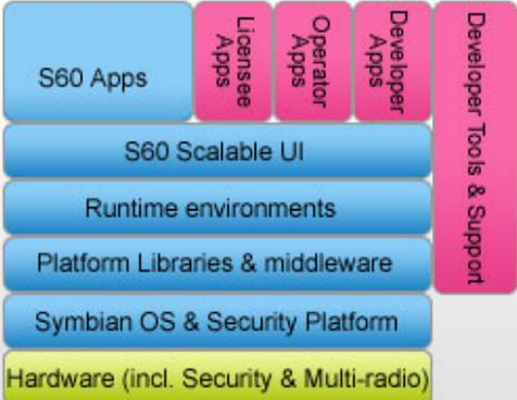
The diagram shows the S60 3rd Edition architecture layers from top to bottom: S60 Apps, S60 Scalable UI, Runtime environments, Platform Libraries & middleware, Symbian OS & Security Platform, and Hardware (incl. Security & Multi-radio). On the right side, there are vertical bars for Licensee Apps, Operator Apps, Developer Apps, and Developer Tools & Support.
