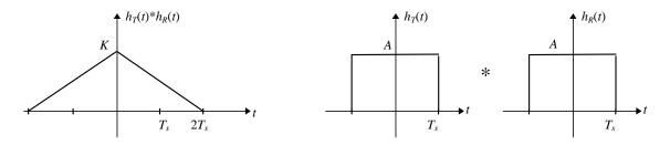
We now only need to find the amplitude *A* in terms of *K*. This can be found by evaluating the convolution integral when the pulses overlap.
