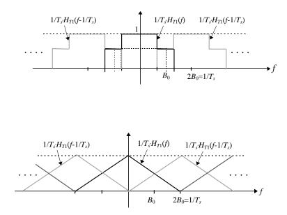
b) When solving for the time-domain waveform it is nice to have a good transformation table that covers most of the Fourier transforms. However, if you are not so familiar with Fourier transforms, here are some different solutions. Let us first study the rectangular spectrum given by the figure below.
