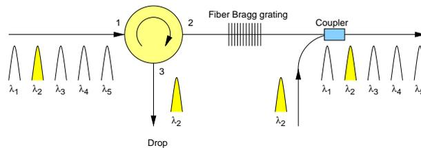
Figure 1: Optical add/drop elements based on fiber Bragg gratings.
