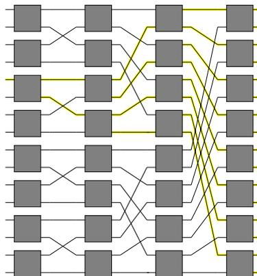
Figure 4:  $16 \times 16$  broadcast star. Each input port is directed to all output ports.
