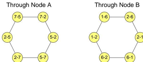
Figure 17: Wavelength assignment problem illustrated for routes routed via WSXC A and B.
