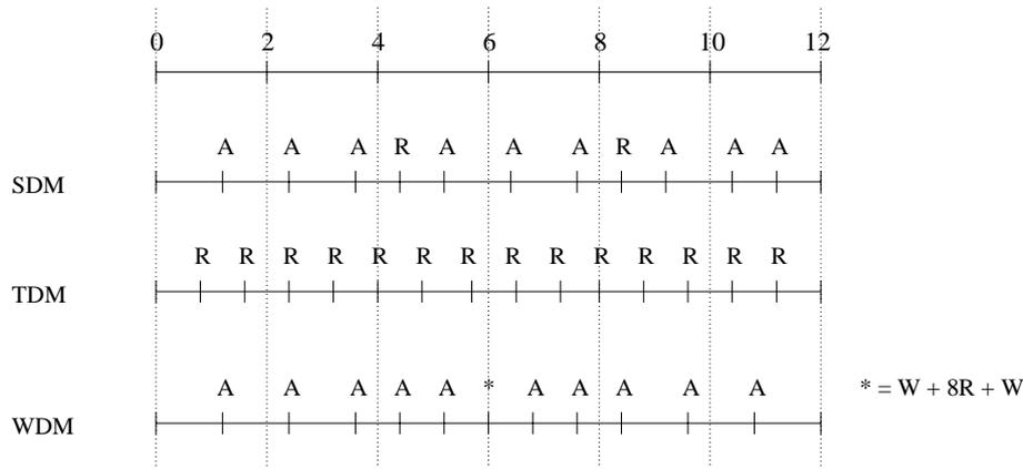
Figure 8: Possible locations of amplifiers and generators in 1200km long link.
