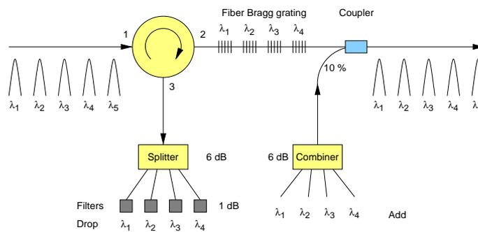
Figure 2: A four-channel add/drop multiplexer architecture.
