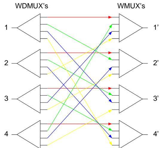
Figure 5: Static  $4 \times 4$  wavelength router.
