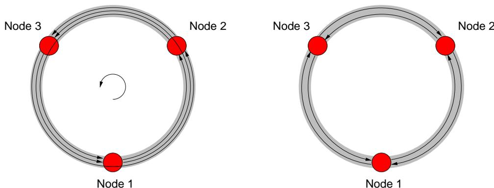
Figure 9: Left figure illustrates the unidirectional ring and the right figure bidirectional ring.
