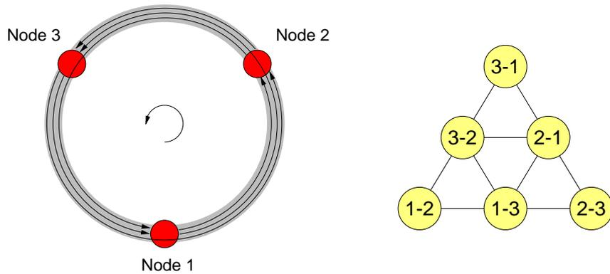
Figure 6: Left figure illustrates the unidirectional ring. The graph on the right shows the corresponding relations between different connections, i.e. which connections must be assigned a different wavelength in order to avoid wavelength conflicts.
