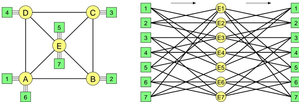
Figure 18: The physical mesh topology and LCH.
