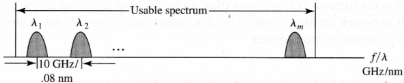
(a)  $\lambda$ -channel Spacing for Separability at Receivers
