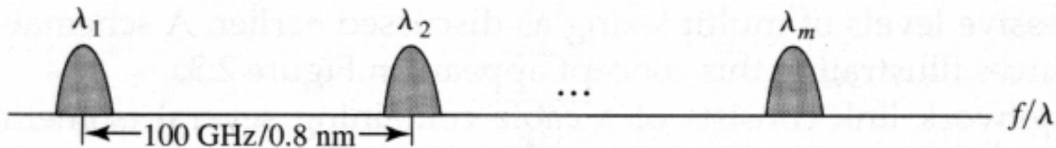
(b)  $\lambda$ -channel Spacing for Separability at Network Nodes
