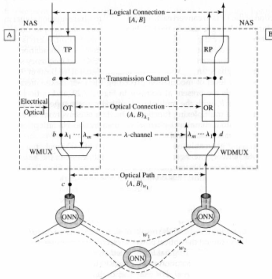
FIGURE 2.30 Example of a logical connection between two NASs.
