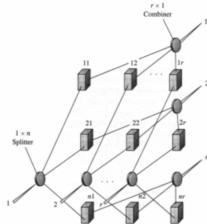
**FIGURE 2.19** Generalized optical switch.
