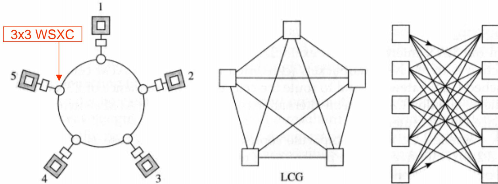
**FIGURE 3.3** Bidirectional ring physical topology.
