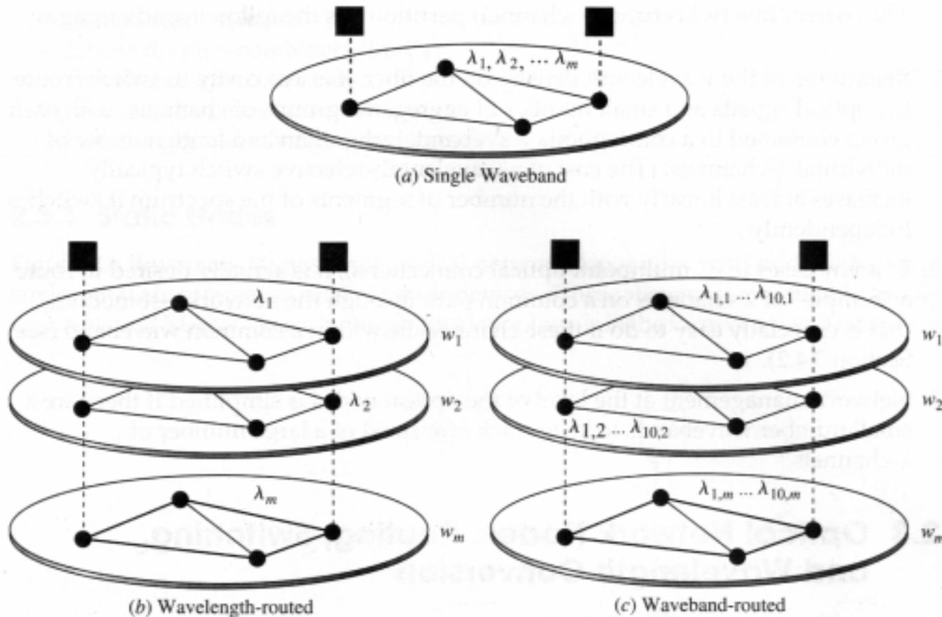
**FIGURE 2.5** Network picture based on spectrum partitioning.
