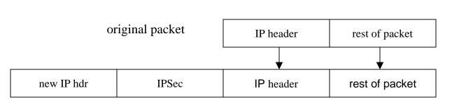
• With ESP everything beyond the header is encrypted => routers and firewalls are not able to look at some fields such as layer 4 ports => Good thing according to security advocates, because fields such as TCP ports should be hidden to avoid divulging information
