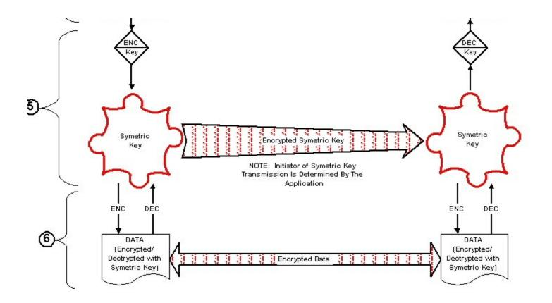
5. Shared secret encrypt a symmetric key and transmit it6. Data encryption and secure communication can occur
