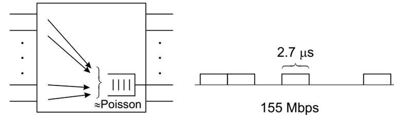
If the link speed is 155 Mbit/s, then the transmission time is  $S = 53 \cdot 8 / 155 \mu s = 2.7 \mu s$ .
