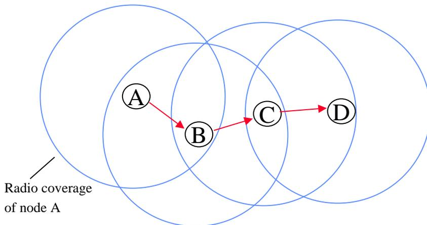
Traffic from A → D is relayed by nodes B and C
