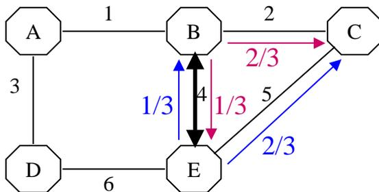
⇒ The packet to X can be sent through Y only if Y is closer to the destination than the current node
