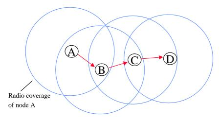
Traffic from  $A \rightarrow D$  is relayed by nodes B and C
