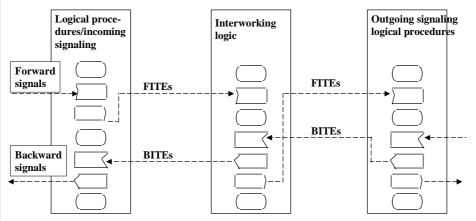
Incoming and outgoing signaling systems are analyzed only to the extent necessary for the specification of interworking. Logic is given using SDL.
