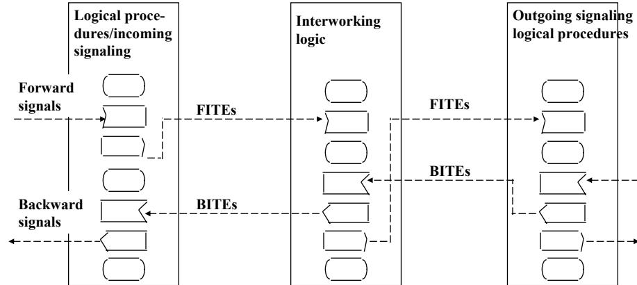
*Incoming and outgoing signaling systems are analyzed only to the extent necessary for the specification of interworking. Logic is given using SDL.*
