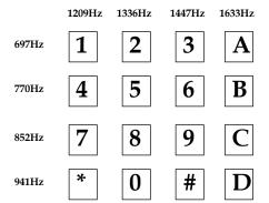
Pushing a button creates a continuous signal with 2 frequences
