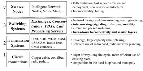
In Circuit networks signaling functionality resides in Switching Systems. In Packet networks (all IP, 3G) signaling resides on Session Layer.
