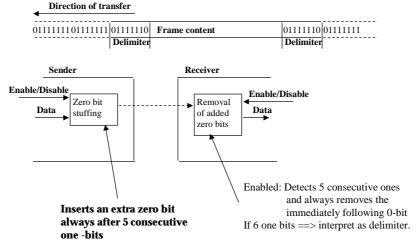
ISDN D-channel layer 2 = LAPD -protocol is based on this HDLC principle. HDLC - High level Data Link Control
