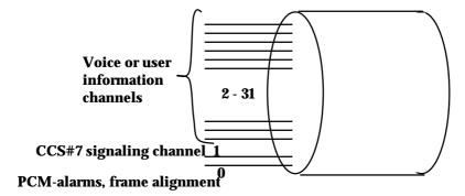
Nowadays, tsl 16 is used for voice! On PCM:s that do not need to have a signaling channel, Tsl-1 may be used for voice or left reserved for signaling for simplicity.
