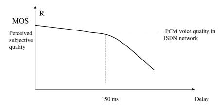
Quality can be measured e.g. based on the E-model or using MOS –measurements. MOS - Mean Opinion Score.
