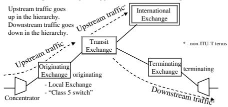
In Addition: *outgoing* traffic, incoming traffic (from the point of view of an exchange Internal traffic: from one subscriber connection to another in a local exchange, terminating traffic: traffic that is terminated to subscribers at a terminating exchange, *transit traffic* = from one network connection to another.
