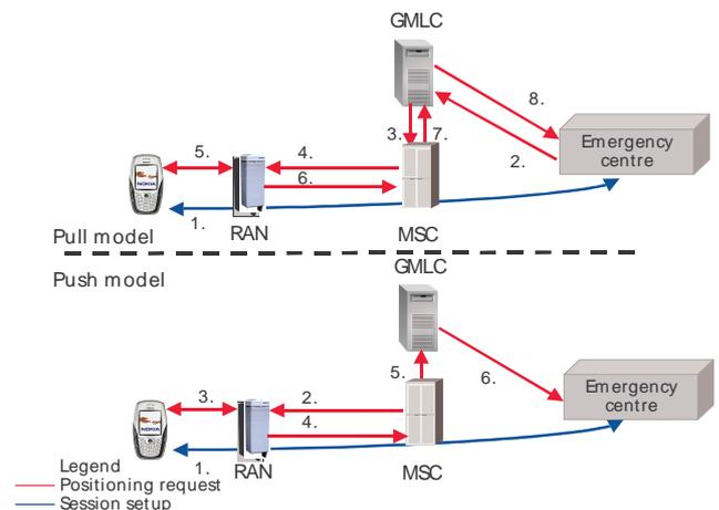
Figure 1. Architecture for pull and push models.
