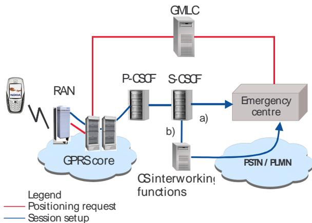
**Figure 2. Architecture for emergency call positioning in the IMS.**
