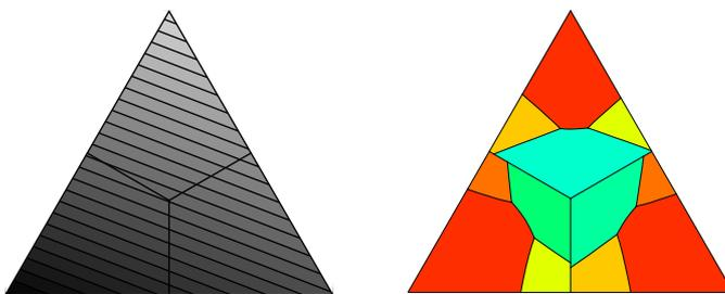
Figure 3.5: Example of inhomogeneous traffic distribution in a cellular system with three base stations (left) and optimal division of the area into sub-areas to be served in different transmission modes (right).
